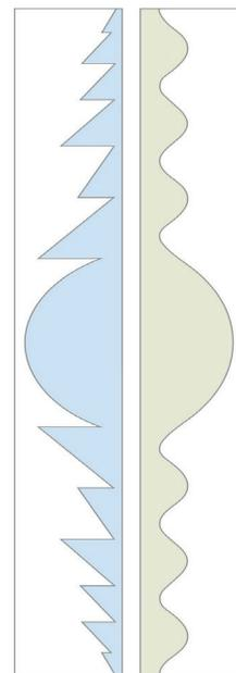
**Figure 1.** Stepless diffractive rings of the Acriva Trinova IOL with a comparison to traditional diffractive trifocal IOL design
