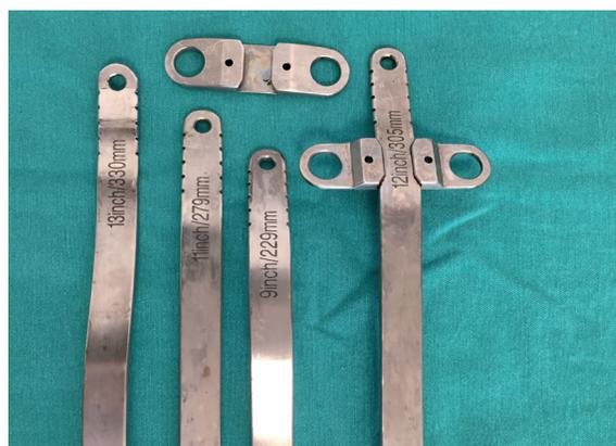
**Figure 1.** Visual of macroscopic surface defects of explanted pectus bars
