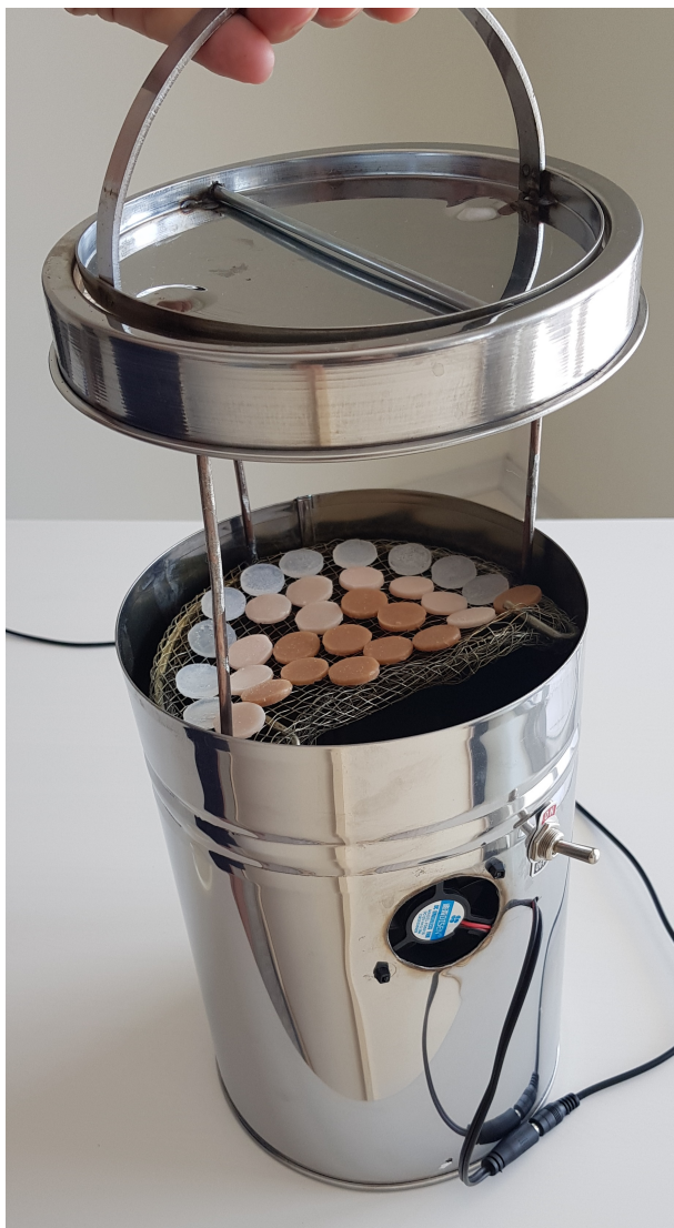
Figure 1. Apparatus used for smoke exposition.
