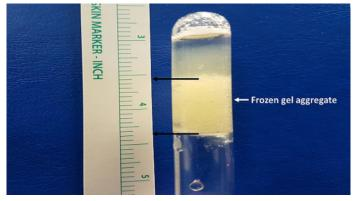
Figure 1. Measurement of the frozen gel aggregate as mm in inverted tube
