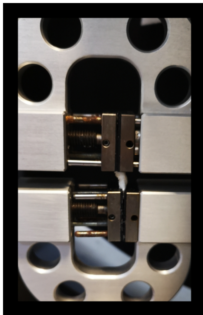
Figure 2. Mounting of the Achilles Tendon Specimen for Biomechanical Testing. Achilles tendon sample clamped between the opposing jaws of the tensile testing machine prior to biomechanical load-to-failure testing.
